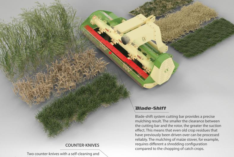
Two counter-knives with a self-cleaning and exchangeable design. These ensure uniform shredding of all of the material. Long material is fed through the rotor in a second step in the crop flow, whereas material that is already shredded passes through. The result is homogenous mulched material.
